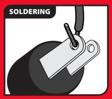
**1.** Insert tinned wire through lug hole before soldering and bend to secure.
