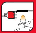
**3.** Wave the flame from a lighter or the tip of a soldering iron near the positioned heat shrink until the wrap constricts to a firm hold. Allow heat shrink to cool.
